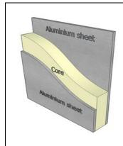
Aluminium composite panels (ACP), made of aluminium composite material (ACM), are flat panels consisting of two thin aluminium sheets bonded to a non-aluminium core. ACPs are frequently used for external cladding or facades of buildings, insulation, and signage.
